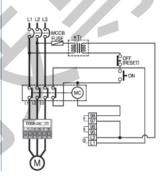
overload, underload, phase loss, phase reversal, phase imbalance, locked rotor, stall TPM-3DE
